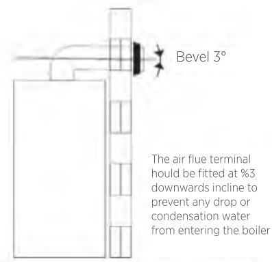
Figure 9 Condensing Heat Only flue slope
